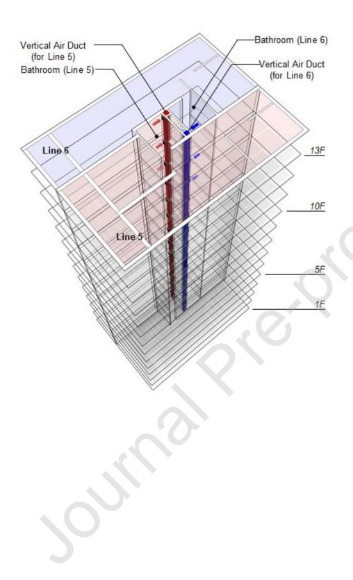
Figure 2. Diagram of the airflow in the air duct
